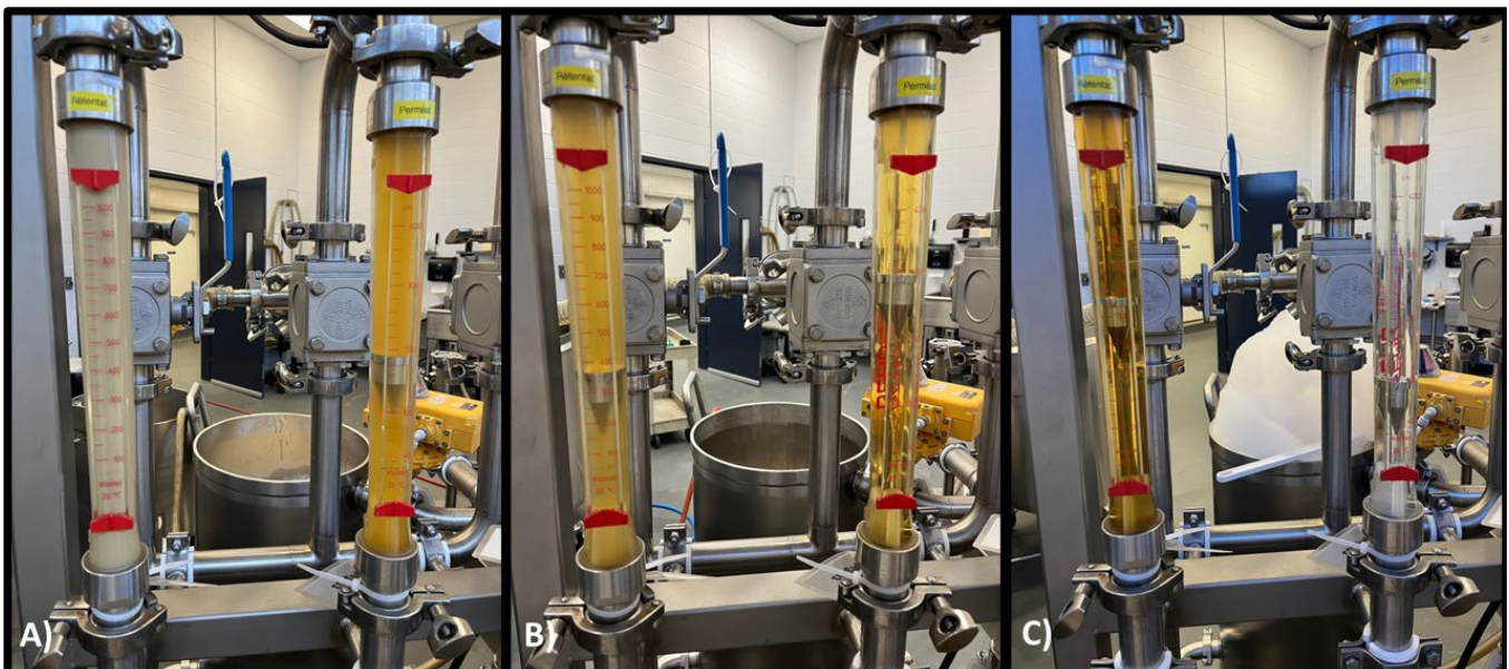
Figure 6. Retentate (left) and permeate (right) after tangential filtration. A) microfiltration ( 0.3\ \mu\text{m} ) to retain fat and particles, B) ultrafiltration to retain large molecules (30 kDa), C) nanofiltration to retain medium size molecules, like peptides (300 Da).
