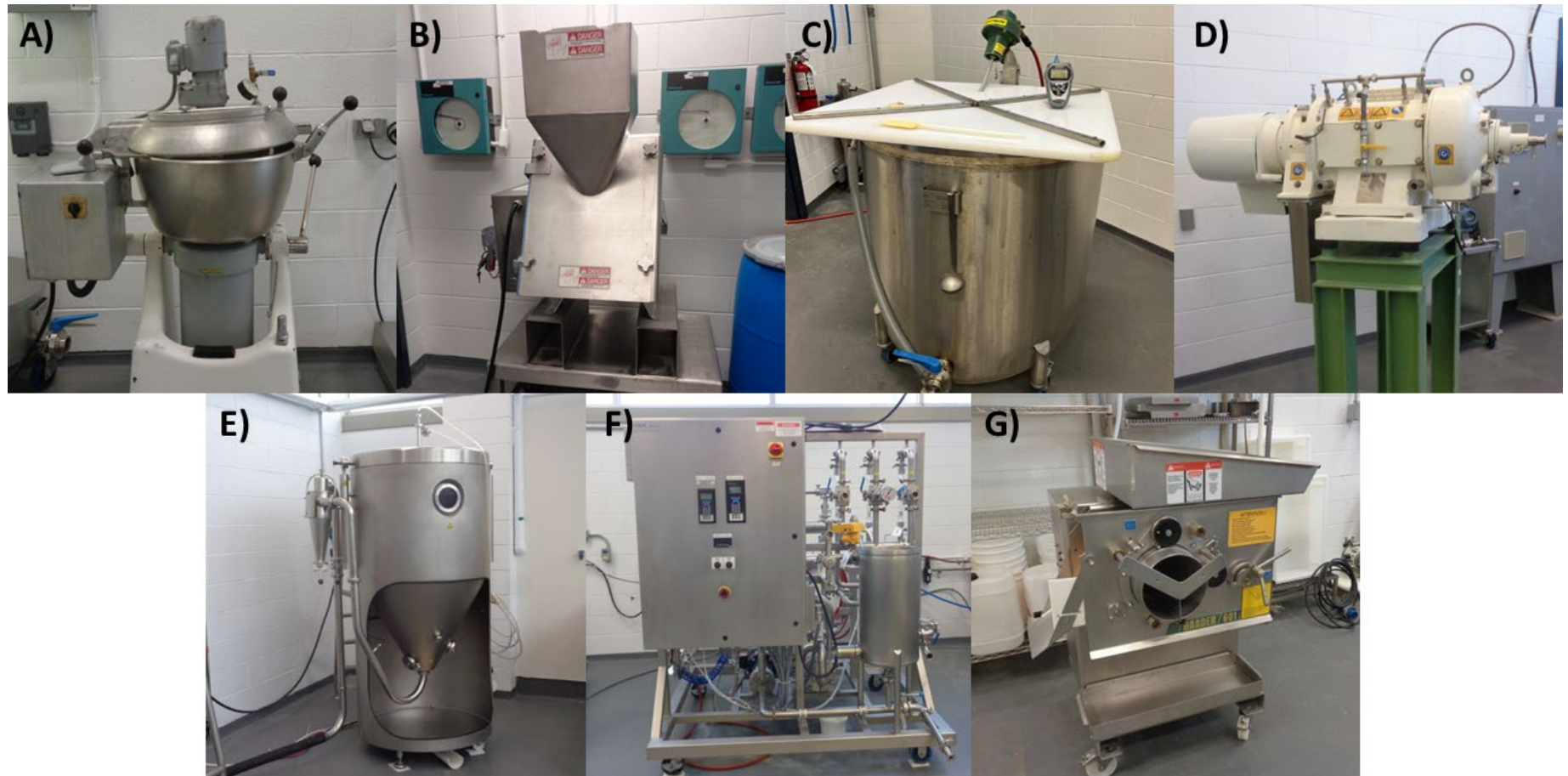
Figure 3. Process equipment used: A) Hobart chopper cutter, B) Comitrol cutter (3 mm crown) C) jacketed hydrolysis tank with stirrer, D) centrifugal decanter for solid removal, E) GEA spray dryer F) tangential filtration unit (only used for isolate production) G) Badger 601 for bone separation, equipped with 1.3 mm drum (not used in hydrolysate preparation)
