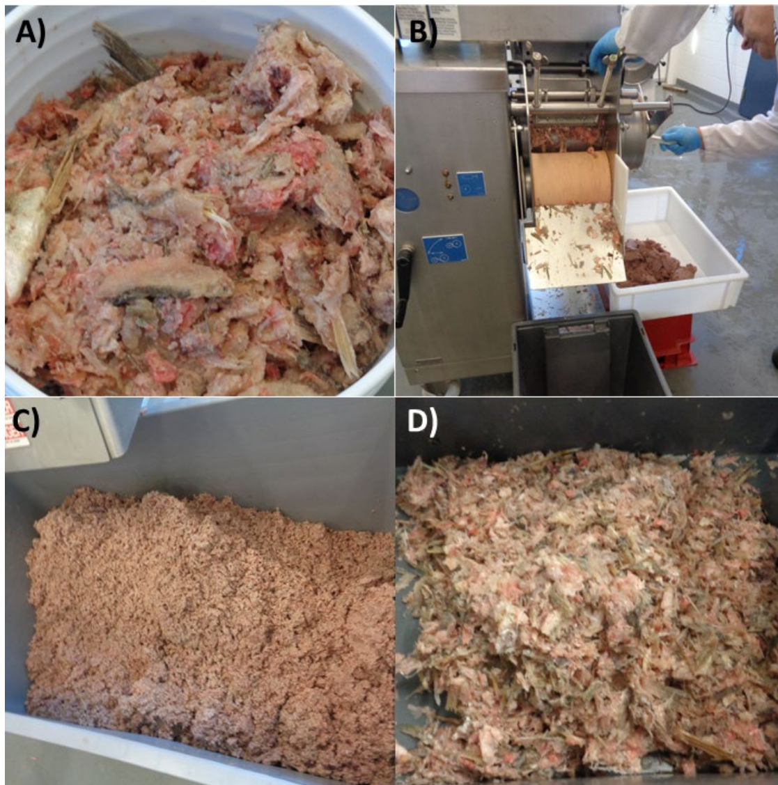
Figure 7. Bone separation experiment during the first pass: A) raw material before processing, B) Baader 601 processing the raw material (1.3 mm separation drum), C) separated meat, and D) mixture of separated bone, fins, cartilages, skin, and scale.
